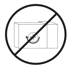
Make sure that you turn the hidden cam a minimum of 190° to a maximum of 210°. Note the position of the arrow on the hidden cam.
